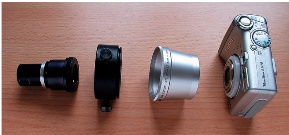
Abb. 1: Von links: Okular, F-Adapter, Filter-Adapter, Canon A520.
